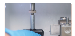
Apply lubricating grease to the tapered part of the spindle chuck
