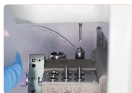
flush the Tool Setter
