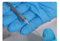
Clean the inner wall of the chuck
