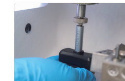
insert it into the spindle chuck
