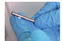
Apply lubricating grease to the tapered part of the spindle chuck
