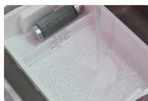
4 Fill the coolant tank with water up to the 2.5-liter mark
