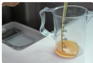
5 Pour 250ml of cutting fluid into coolant tank
