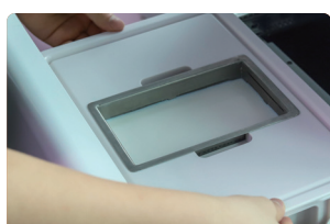
7 Place the coolant tank back into the machine and tighten it securely
