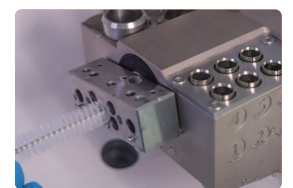
Clean the work area with a pipe brush
