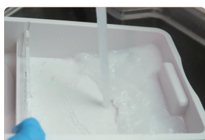
3 Use clean water to flush and clean the coolant tank
