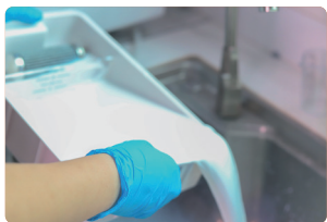
1 Empty the old cutting fluid
